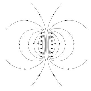
**Fig. 6.23** A uniform current-carrying plane surface
