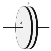
Fig. 2.13 Parallel-plate capacitor
