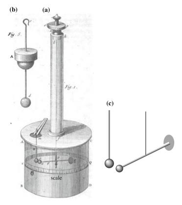
Fig. 1.2 Coulomb's torsion balance experiment. a the apparatus, b detail showing the fixed sphere; both are from the memoire, c torsion balance detail, showing the crossbar, charged spheres and counterweight
