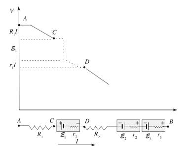
Fig. 5.18 A circuit section and the voltage across it
