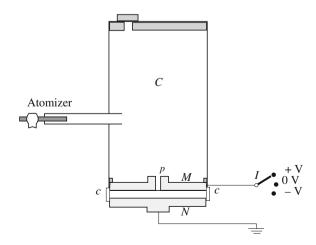
An intense light beam enters and exits through two small glass windows c through the volume in which the drop that has gone through the hole is moving. The drop is observed with a telescope through a third small window (not shown in the figure) at  $90^{\circ}$  with the light beam. The droplet scatters some light and appears to the experimenter as a bright star in a dark field.
