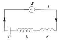
L and a capacitor (or condenser) of capacitance C. To find the equation governing this circuit, let us consider having a unit charge going about the full circuit. Its final energy is equal to the initial one. We shall then express in a formula the fact that the sum of the work done on the charge is zero.
