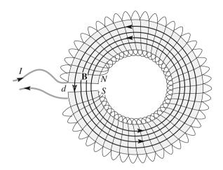
Electromagnets are used to produce the magnetic field of requisite intensity in the useful space region, as we already did on several examples. We can start again from Fig. 9.17 (the torus must now be thought of as being much larger and heavier than for an inductor). The core must be interrupted to make the useful space available. Let us cut a short gap, of thickness d, as in Fig. 9.19, creating two magnetic poles, a North one and a South one. Such systems are called dipole magnets.
