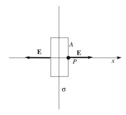
**Fig. 1.23** The field of two parallel oppositely charged planes
