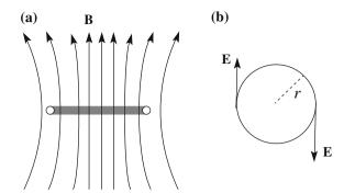
was called a betatron. Betatrons accelerate charged particles, typically electrons (hence the name), up to quite high energies. We are mainly interested here in the working principles, and we shall consequently ignore all technical details.
