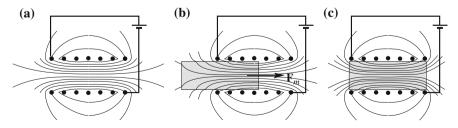
Fig. 9.27 a A solenoid in a vacuum, b introducing the magnetic material core, c the core is completely inside
