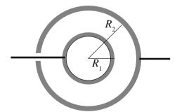
**Fig. 2.16** Geometry of a cylindrical capacitor
