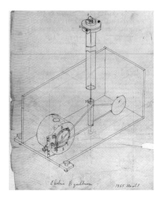
The main electric components of the apparatus were two batteries, a large one to provide the high voltage between the disks and a small one to provide the current to the coils, a calibrated resistor *R* and a galvanometer.
