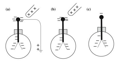
Fig. 2.4 Charging an electroscope by induction
